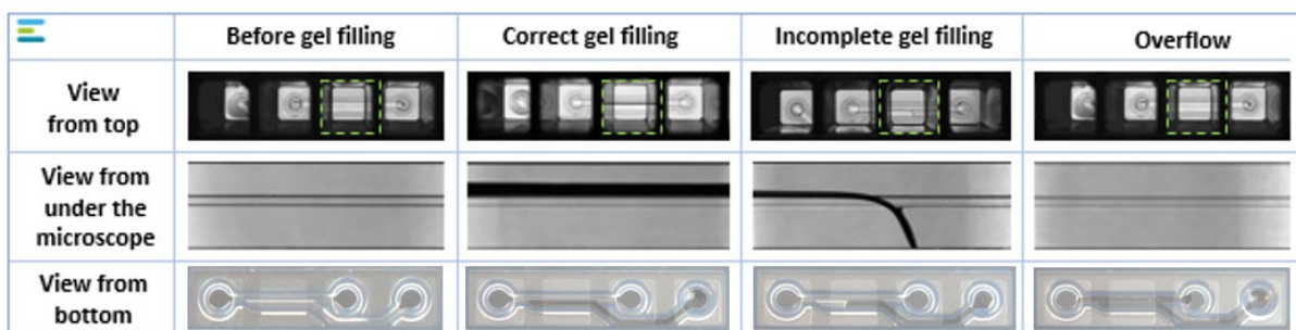
Figure 5: Overview of correct gel filling, incomplete gel filling, and overflow in the OrganoPlate® 2-lane
